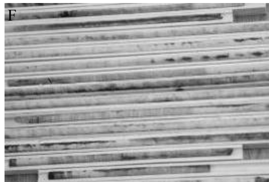
Figure 5. 10 Mounting cores. Once the cores have been dried, they are mounted on prefabricated wooden core mounts with water soluble white glue. The information from the straw is written on the side of the core mount (A). A thin bead of glue is extruded into the groove (B). The core is delicately removed from the straw and pressed into the groove (C). The core is then secured to the core mount to keep it from curling as it absorbs the moisture from the glue (D). The string can be tied off and the mount should sit for at least two hours before it can be sanded (E). Once the string is removed all of the cores are ready for sanding (F). String, tape, binder clips, or weights can be used to hold the cores in place while the glue dries (photos by Jim Speer).
