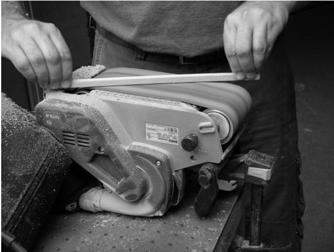
Figure 5. 13 Sanding cores. Cores can be sanded on a belt sander (4 X 24" belt sander recommended for the surface area that it provides) with progressively finer grits (50, 120, 220, 320, and 400 grits) to polish the cross sectional view until the individual cells are apparent under a microscope at 40X magnification. In this picture the operator is sanding the core at a 45 degree angle from the axis of the sander so that he can see the striations made from the previous grit. Once those striations are sanded off of the core, it is time to move on to the next finer grit. Repeated visual examination of the core helps determine when the core has been sanded enough. Of course, the final test is to examine the core under the microscope (photo by Jim Speer).
