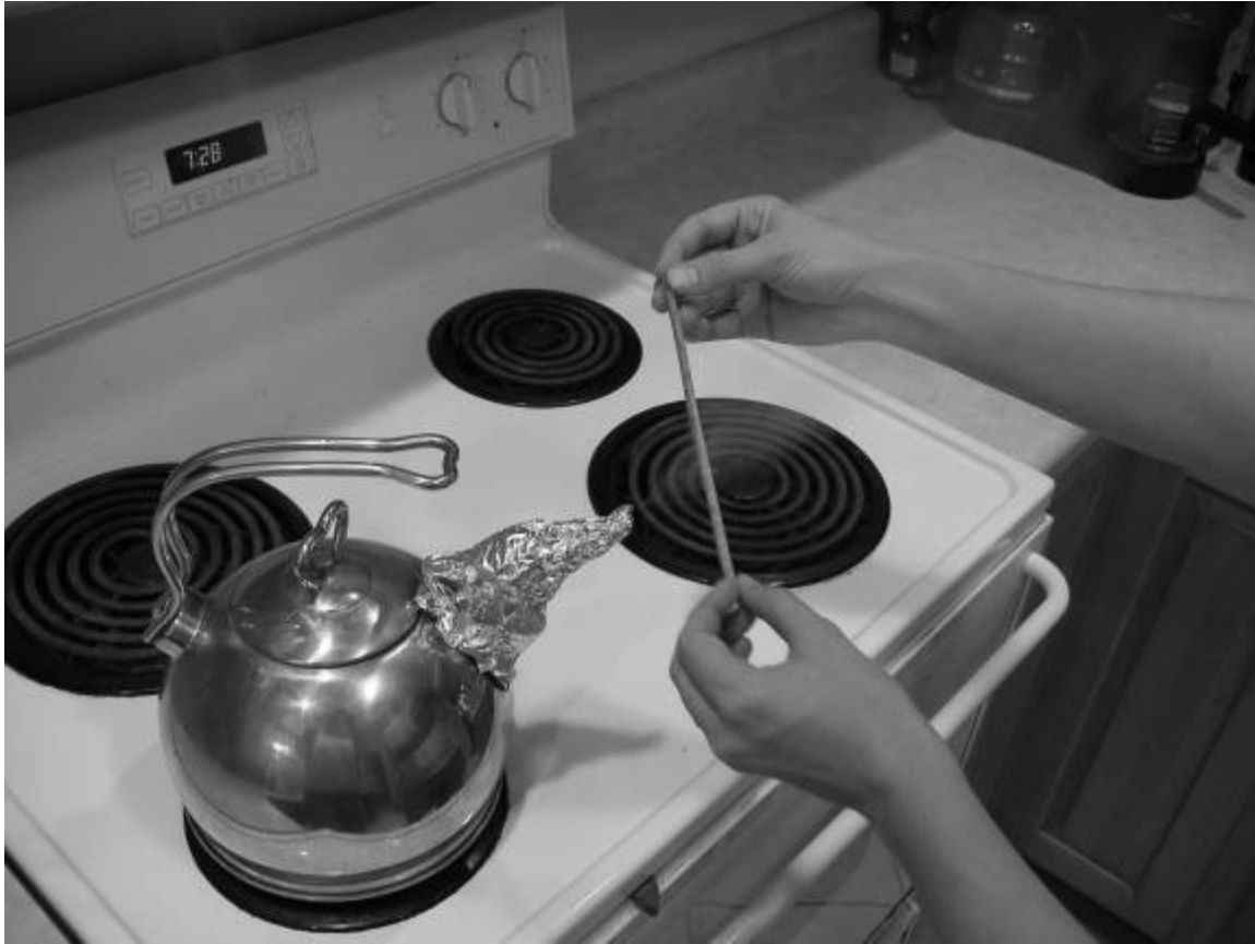
Figure 5. 11 Untwisting cores. If a core is twisted (usually due to a nicked or dull increment borer), then the cores can be straightened over a jet of steam (photo by Jim Speer).
