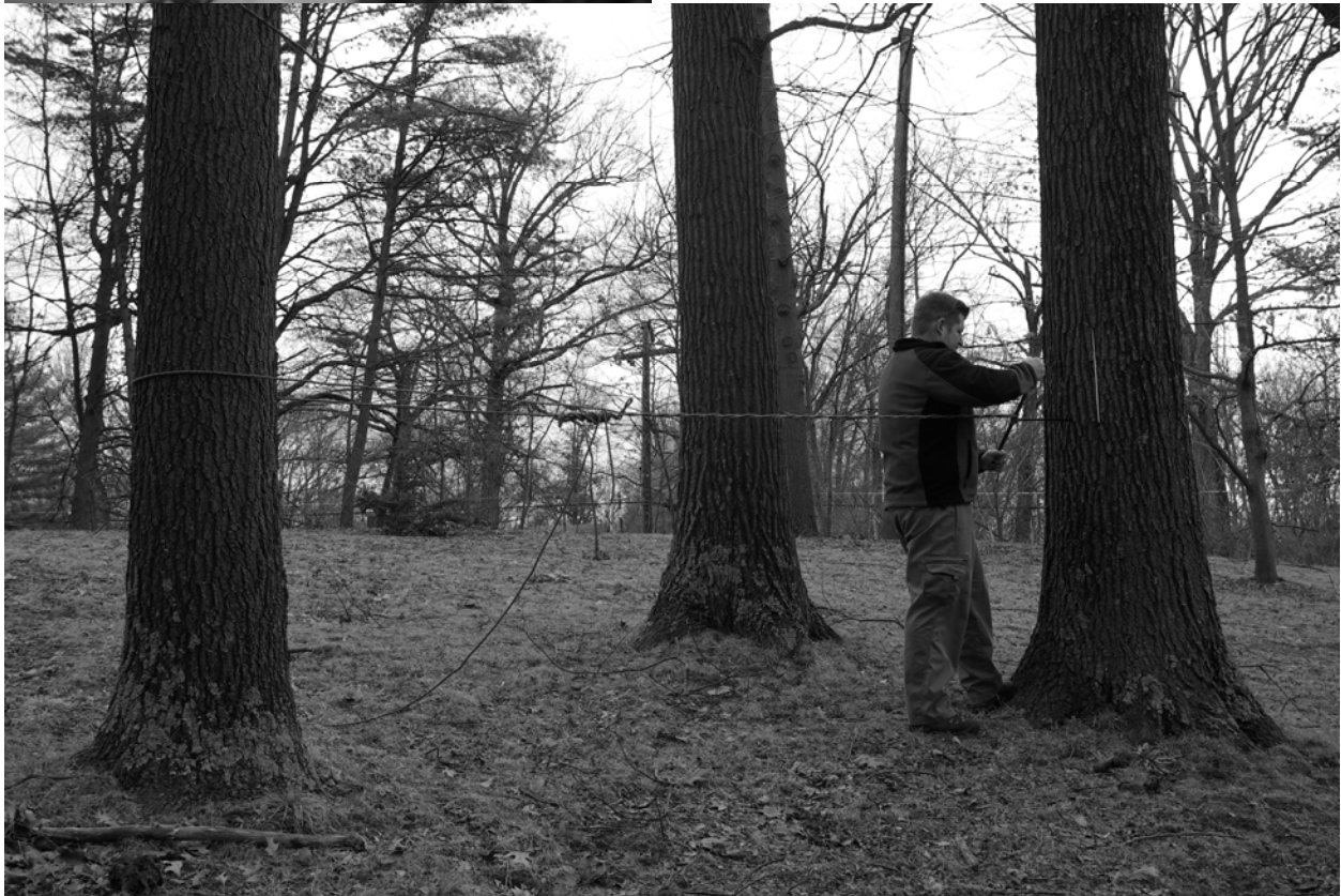
Figure 5. 7 Spanish windlass. The Spanish Windlass technique uses the force generated from a twisting rope to provide backward pull on the increment borer, enabling you to remove a stuck borer from a tree. You need to connect the rope around the handle of the increment borer and a tree directly in line with the increment borer, then twist the handle of the borer counterclockwise. The increment borer will come out of the tree quickly when most of it has been rotated out of the tree, so be careful with this technique. You should keep a tight grip on the borer to control it as it comes out so that you or the borer does not get hurt.
