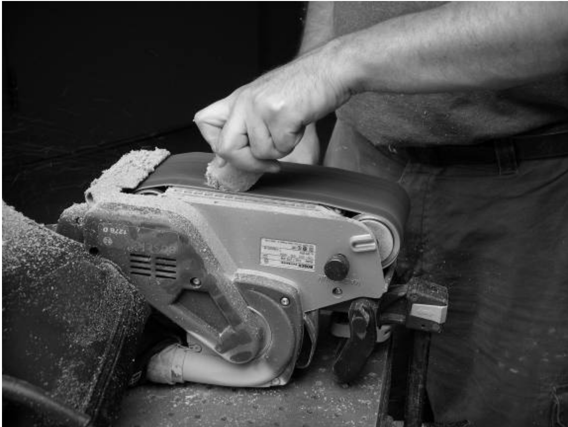
Figure 5. 14 Cleaning a sander belt. Sander belts lose efficiency before the grit is worn down as they become covered in a layer of resin and dust from the wood. You can clean sander belts using a rubber gum eraser that can be purchased at most woodworking stores. The eraser pulls the saw dust from within the grit of the sandpaper and clumps it together, shooting it from the sander. If cleaned, sander belts can be re-used some 20 or more times before the grits wear down (photo by Jim Speer).
