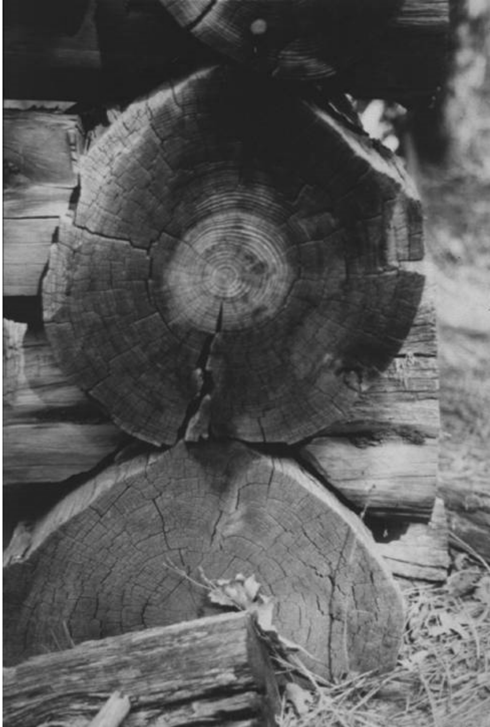
Figure 7. 14 Cross section of a beam from a log cabin. Many pioneer log cabins have very old wood incorporated in their structures. Some of these beams can prove problematic in determining accurate outside dates because the outer rings were often removed as the timbers were shaped for construction. Care must be taken to sample through an area that has complete outer rings as observed in the cross section (photo by Jim. Speer).
