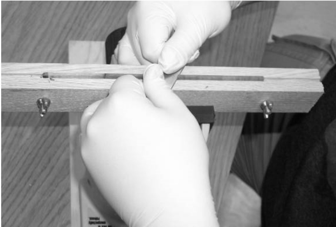
Figure 11. 1 A dendrochemistry sample in a core clamp. The clamp is constructed from two pieces of wood that are grooved on the top center to hold the core. They are drilled through the center of the two boards in three places and a bolt with a wing nut is inserted through each hole to clamp down the core. In this picture, note that the researcher wears gloves to avoid contamination of the sample and uses a razor blade instead of sandpaper to surface the sample prior to dating (photo by Jim Speer).
