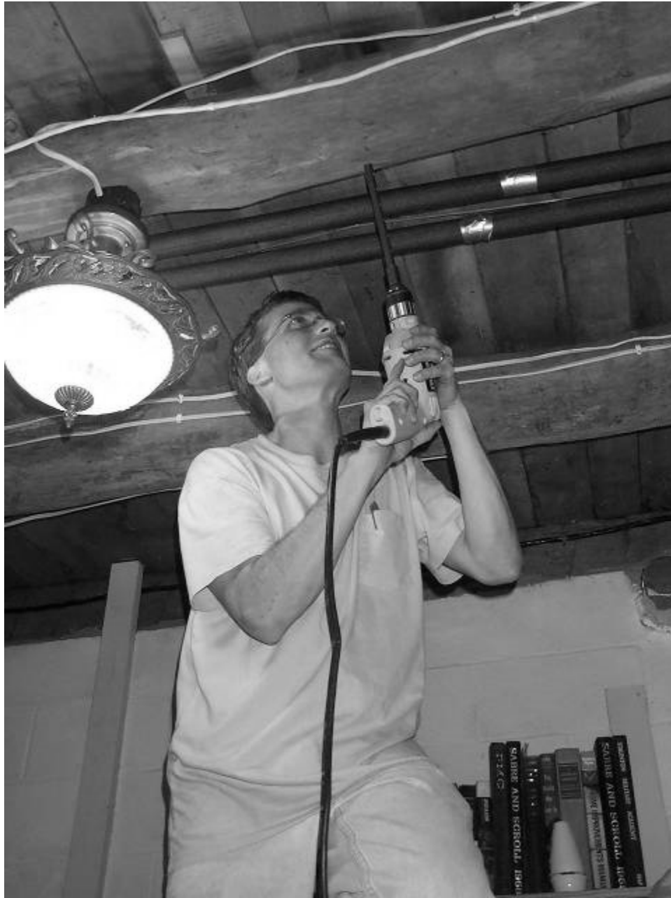
Figure 7. 8 An Archaeological borer. An archaeological drill can be used to cut a 12 mm core from dry wood. This archaeological borer uses a hollow bit that cuts away the wood around the core as the bit is drilled into the beam. A starter plate can be used to hold the bit in place while the core is taken. A long piece of metal is inserted along the side of the core, and then twisted to break the core off on the inside of the beam. This tool is being demonstrated by Dr. Darin Rubino (photo provided by Darin Rubino).
