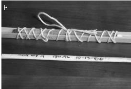
Figure 5. 10 Mounting cores. Once the cores have been dried, they are mounted on prefabricated wooden core mounts with water soluble white glue. The information from the straw is written on the side of the core mount (A). A thin bead of glue is extruded into the groove (B). The core is delicately removed from the straw and pressed into the groove (C). The core is then secured to the core mount to keep it from curling as it absorbs the moisture from the glue (D). The string can be tied off and the mount should sit for at least two hours before it can be sanded (E). Once the string is removed all of the cores are ready for sanding (F). String, tape, binder clips, or weights can be used to hold the cores in place while the glue dries (photos by Jim Speer).
